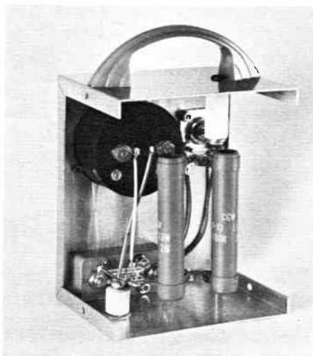
fig. 35. Inside the wattmeter, showing the CGW "R Series" resistors.
