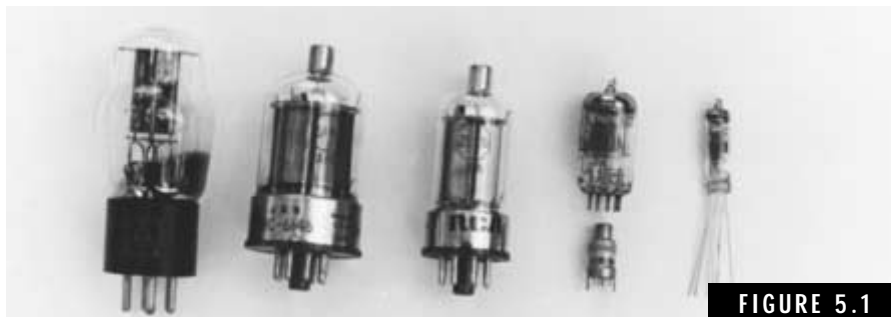
Typical receiving and transmitting vacuum tubes.
